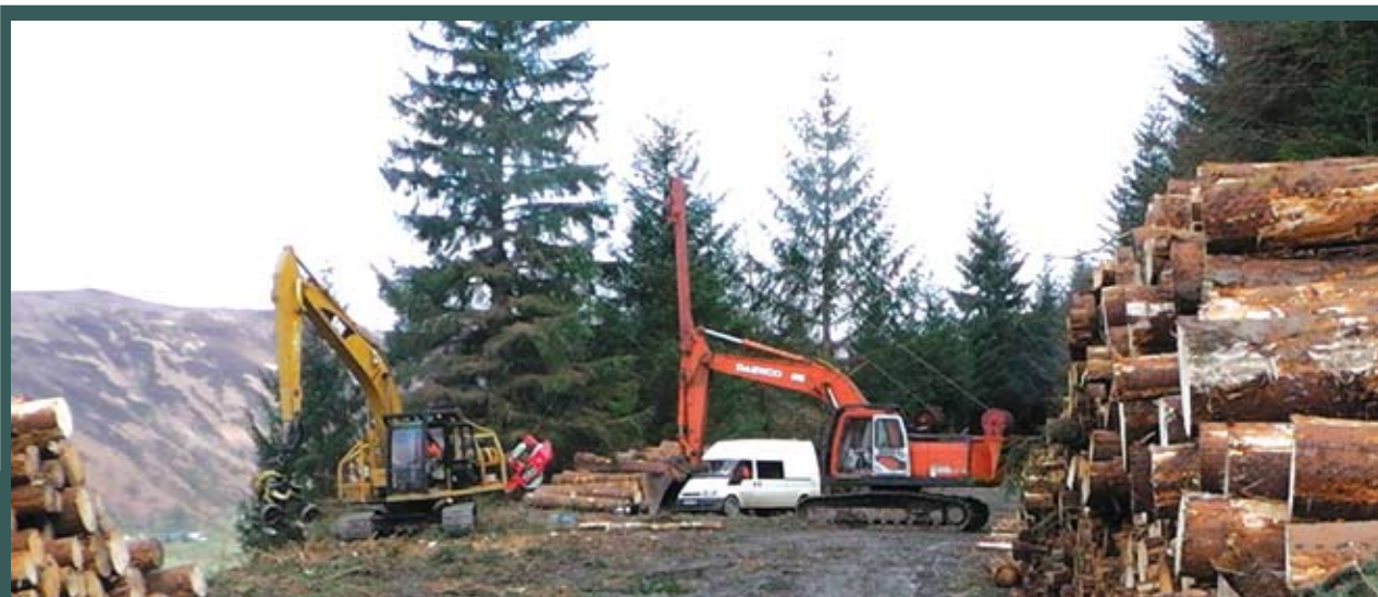
The Daewoo 220 Solar excavator skyline moved back to allow the Cat 320CL harvester to operate.
