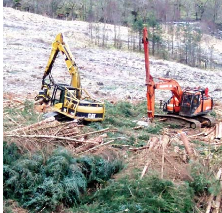
The Daewoo 220 Solar excavator skyline and the Cat 320CL harvester working in tandem at Glen Creran.
