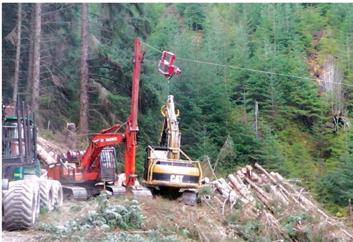
Everything in harmony on the landing – the Daewoo 220 Solar excavator skyline with the Koller USKA 1.5 carriage, the Cat 320CL harvester and the John Deere 1410D forwarder.
